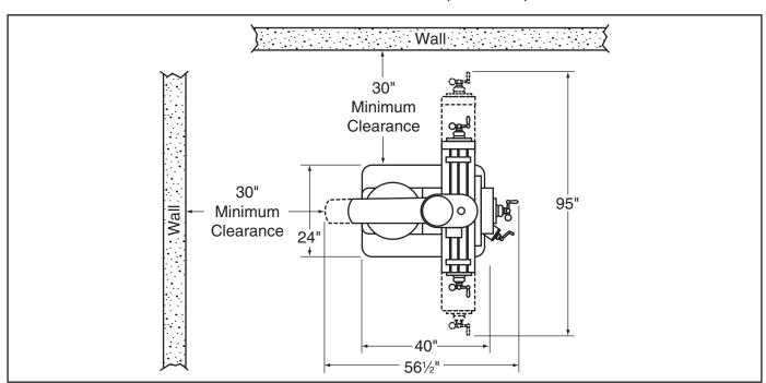
Figure 4. Minimum working clearances.
